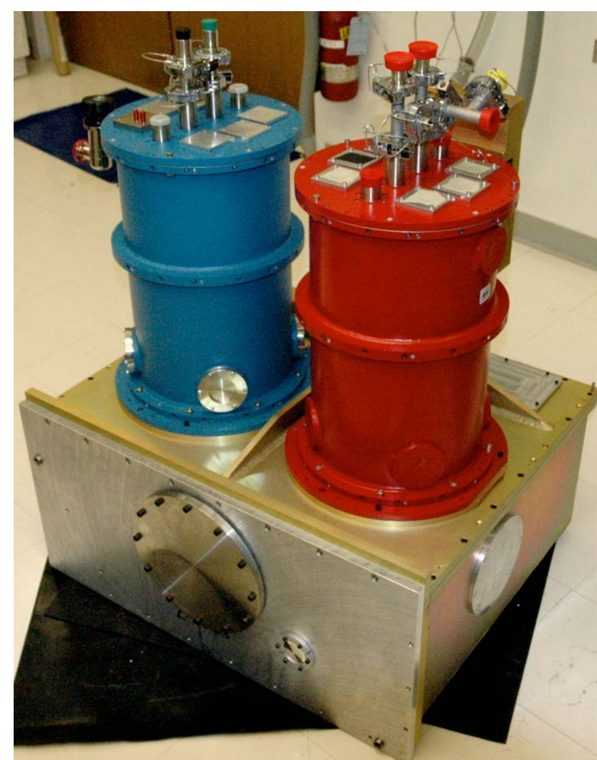
Above: CASIMIR flight cryostats mounted on the optics box. At frequencies below 1 THz, the mixers will operate at 4 K. For the higher frequency bands, the LHe bath will be pumped to operate the mixers at 2.5 K.
